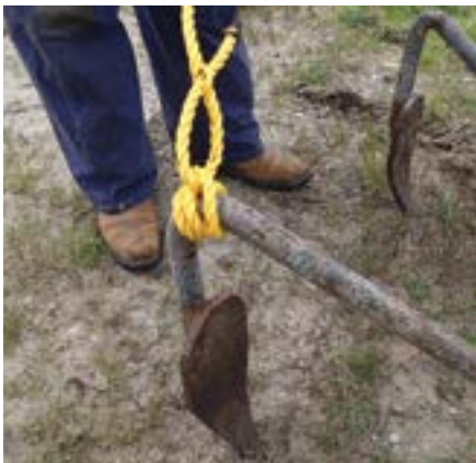
Joel Petersen, captain of the Joy , demonstrates how to tie ropes to trap net anchors, May 2017. Setting each trap net in Lake Michigan requires up to ten anchors. PHOTOS BY RAQUEL JIMENEZ
